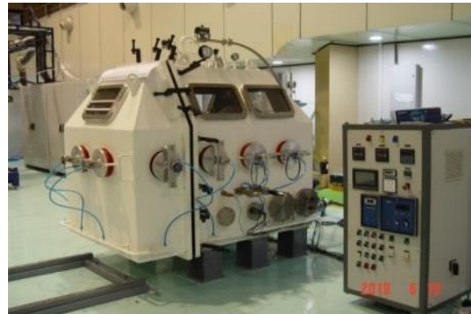
Welding Glove-box for Cavity Dressing
