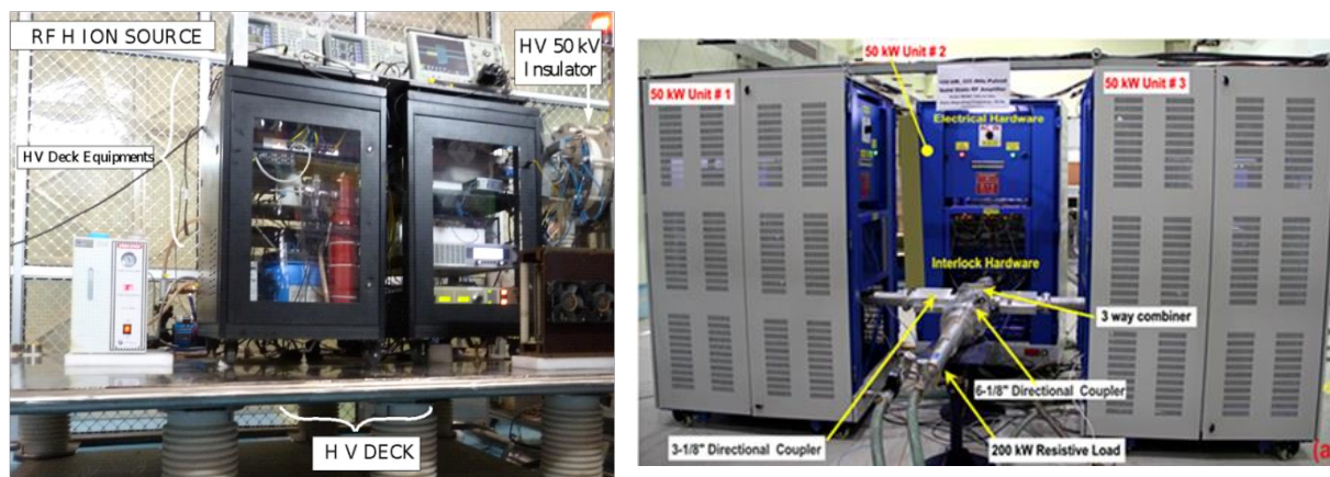
Fig. 4.4.1: RF discharge based H- ion source (left) and 325 MHz, 150 kW Solid State Amplifier (right) developed at RRCAT.
