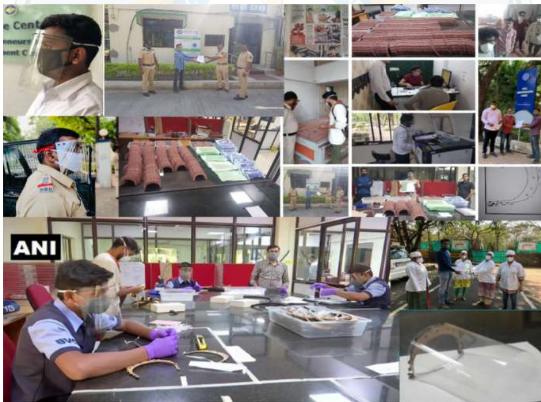
The face shield comprises of a transparent clear polyester sheet that protects the face from any airborne fluid particles. The sheet is kept in place with the help of a headband and an elastic strap. The face shield design uses MDF and can be machined (instead of laser cutting), which makes the process simpler, cheaper and scalable.
