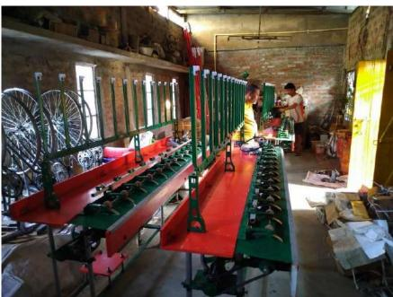
Figure 27: Hank to Bobbin yarn winding machine
