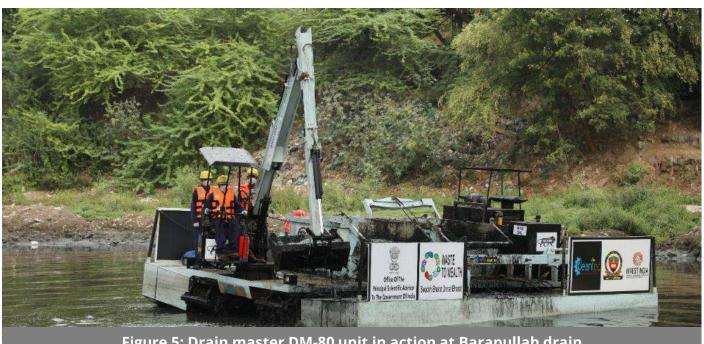
Figure 5: Drain master DM-80 unit in action at Barapullah drain
