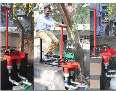
Figure 23: Treadle pump under demonstration in Sarjapur, Bangalore
