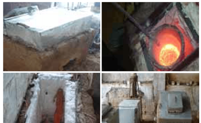
IIT Delhi developed and tested natural-draft LPG-fired metal-melting and mould-heating furnaces (Image Credits: IIT Delhi)
