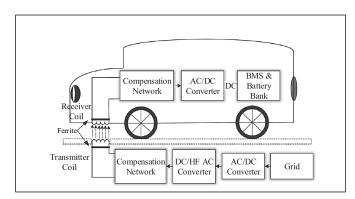
Figure 6: Block Diagram of Wireless Charging System
