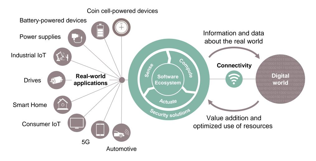
Sense: sensors Compute: microcontrollers, memories Actuate: power semiconductors Connectivity: Wi-Fi, Bluetooth, USB
