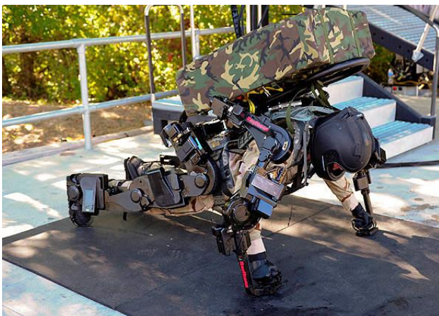
Figure 15: A soldier performing push-ups with the XOS 2, a second-generation robotics suit developed by Raytheon for the US Army as part of Defence Advanced Research Project Agencies, 'Human Performance Augmentation' programme.
