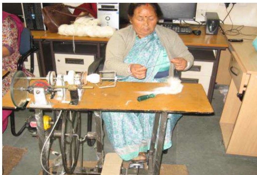
Figure 26: Modified Bageshwari wool charkha developed by RuTAG IIT Roorkee
