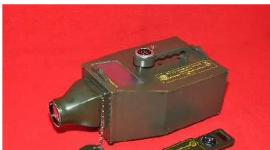
Figure 46: Preemptor MK-II, RBS technique based explosive detector developed by IRDE, DRDO
