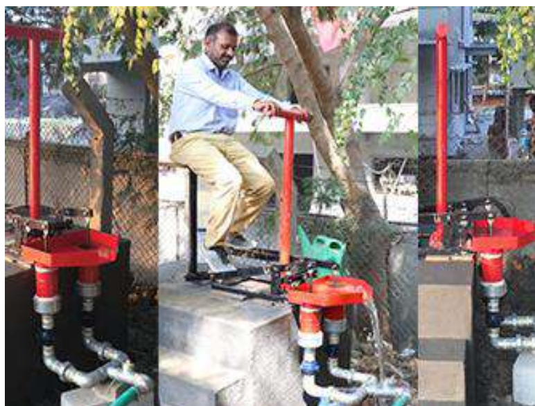
Figure 23: Treadle pump under demonstration in Sarjapur, Bangalore
