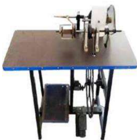
Figure 26: Modified Bageshwari wool charkha developed by RuTAG IIT Roorkee
