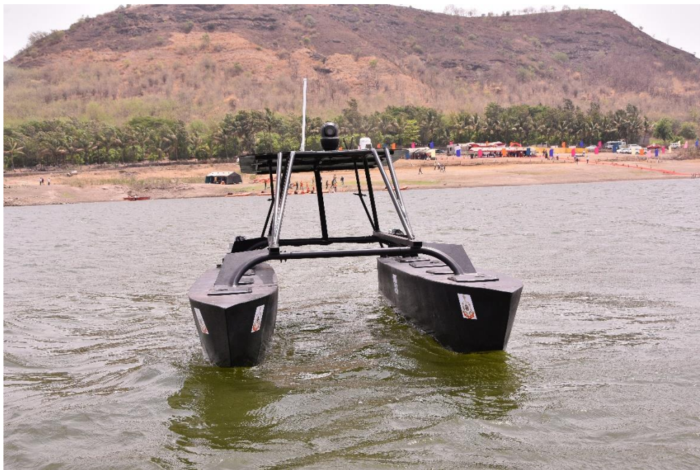
Figure 28: (A) Side view of the UMSV; (B) Front view of the UMSV, Catamaran Hull design
