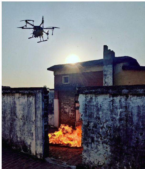
Figure 19: Payload drone with 15L water tank was tested for dynamic firefighting capabilities
