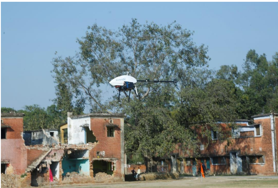
Figure 16: Battery-powered Fully Autonomous Unmanned Helicopter with Day/Night Camera (40x Zoom)
