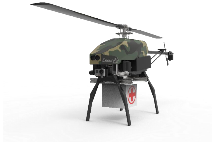
Figure 35: Twin Rotor VTOL UAV with Payload and Surveillance capabilities (Representative Image)
