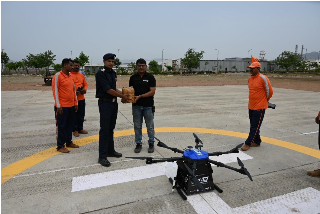
Figure 22: Pre-programmed fully autonomous drone flight with 4kg custom payload was carried out from Jadhavwadi dam to 5BN HQ, Sudumbre (approx distance of 3km)
