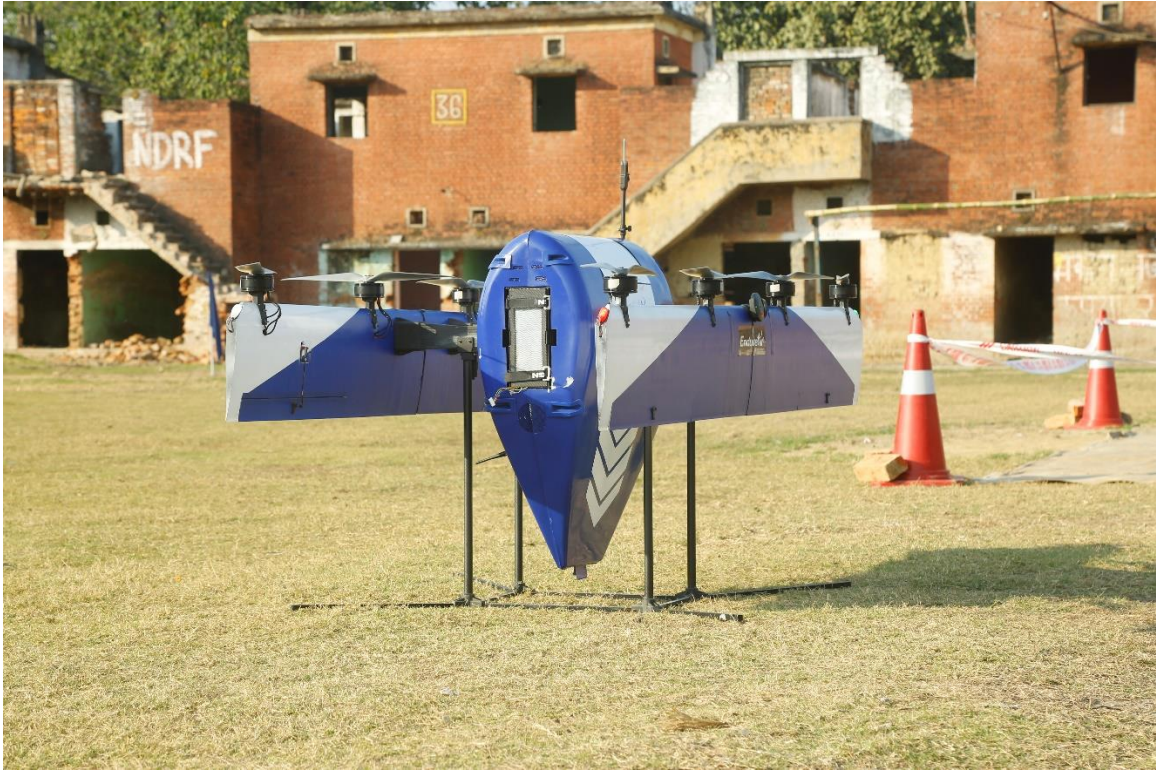
Figure 18: Hybrid VTOL design Logistics drone (~5kg payload)
