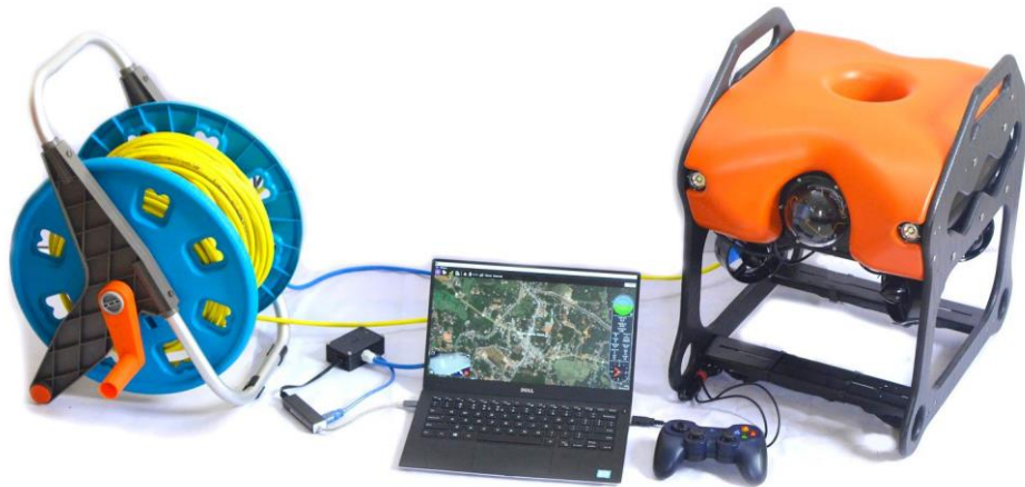
Figure 32: Sample images of Imaging SONAR, dehazed video feed from the ROV, ROV + Control Station + Tether
