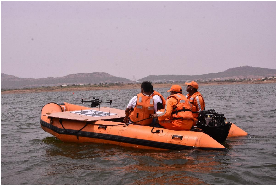
Figure 34: UAV performing a dynamic landing on a moving rescue boat, in a fully autonomous mode
