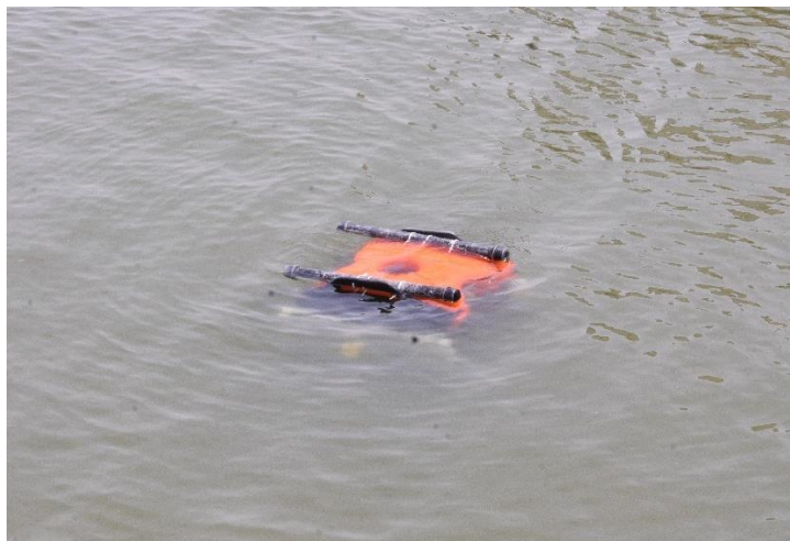
Figure 30: Tethered ROV being deployed underwater for a dummy human body detection exercise
