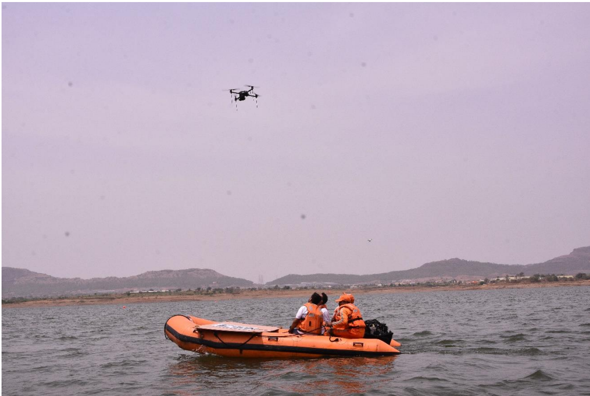
Figure 33: Autonomous UAV preparing for an approach to the rescue boat with landing pad
