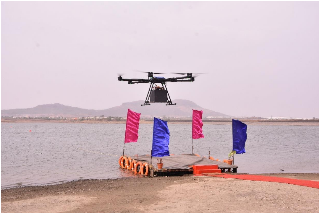
Figure 21: Manual flight of payload drone strapped with 4kg payload was carried out at test site, 5BN
