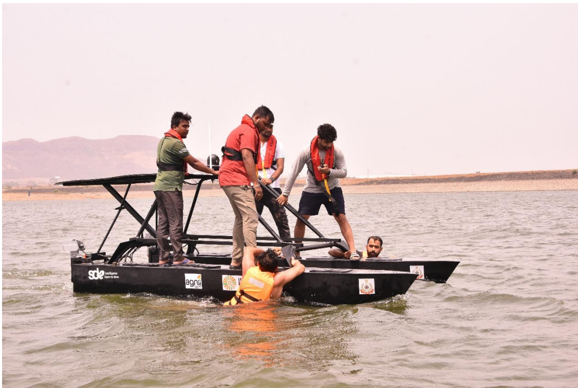
Figure 29: (A) The UMSV cruising at 4-5 knots in Jadhavwadi Lake; (B) Payload carrying capacity being demonstrated; 6 adults were onboard with slow movement.
