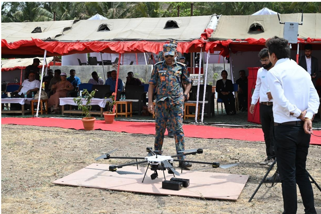
Figure 20: Fully autonomous payload drone (5kg capacity) with extended range (20km)
