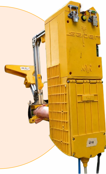
SAPER, automated coconut sap tapping robot
