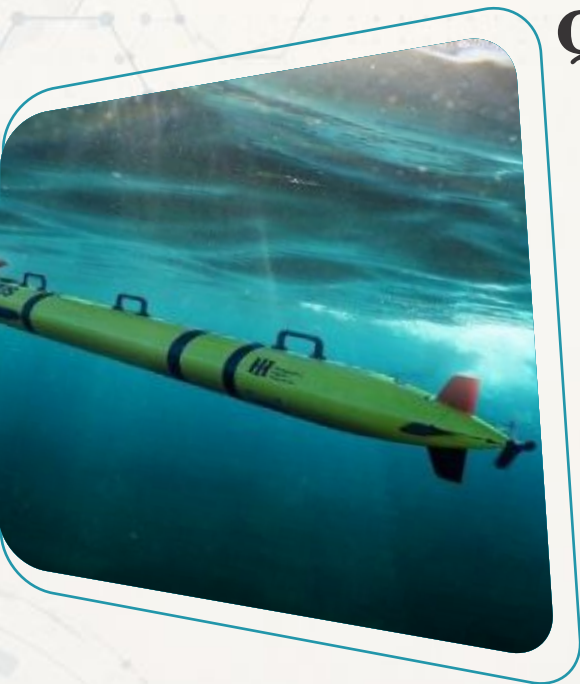
Man-portable Autonomous Underwater Vehicles (MP-AUVs) for naval mine countermeasure missions | Photo: DRDO
